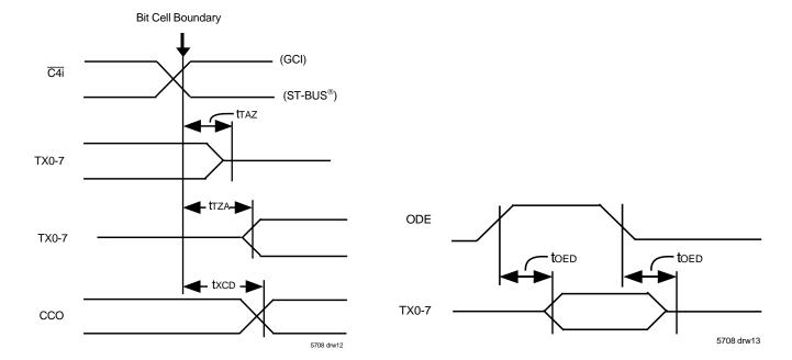
Figure 9. Serial Outputs and External Control
