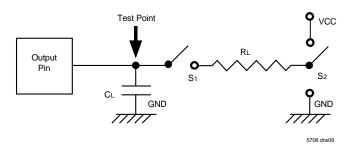
Figure 6. Output Load
