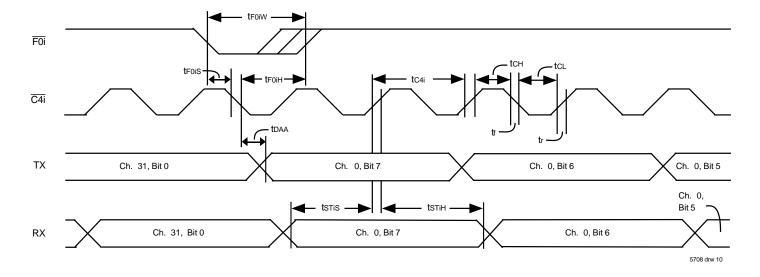
Figure 7. ST-BUS® Timing
