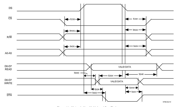
Figure 11. Motorola Non-Multiplexed Bus Timing
