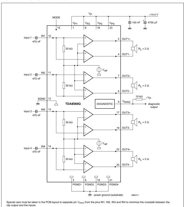
To avoid switch-on plops, it is advised to keep the amplifier in the mute mode for a period of ≥150 ms (charging the input capacitors at
