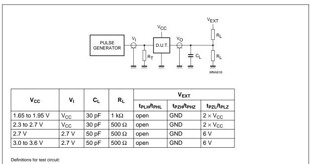
R<sub>L</sub> = Load resistor.
