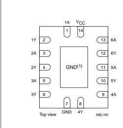
(1) The die substrate is attached to this pad using conductive die attach material. It can not be used as a supply pin of input.
