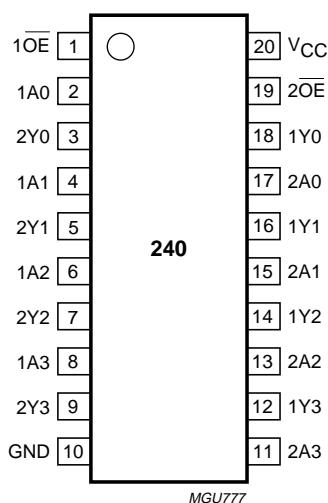
Fig.1 Pin configuration SO20 and (T)SSOP20.
