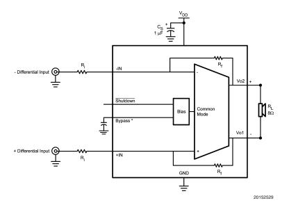
FIGURE 1. Typical Audio Amplifier Application Circuit
