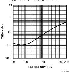
THD+N vs Frequency  $V_{DD} = 3V$ ,  $R_L = 4\Omega$ ,  $P_O = 225$ mW
