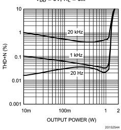
THD+N vs Output Power  $V_{DD}$  = 5V,  $R_L$  =  $4\Omega$
