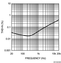
THD+N vs Frequency  $V_{DD} = 5V, R_{L} = 4\Omega, P_{O} = 1W$
