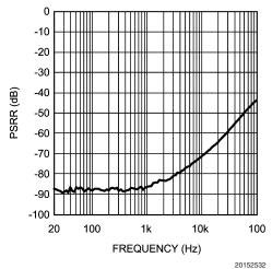
PSRR vs Frequency  $\label{eq:VDD} {\rm V_{DD}} = 3{\rm V}, \, {\rm R_L} = 8\Omega$  Inputs terminated to GND, BW = 500kHz
