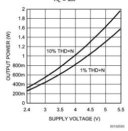
Output Power vs Supply Voltage
