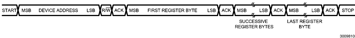
FIGURE 8. Multi-Byte Write Example
