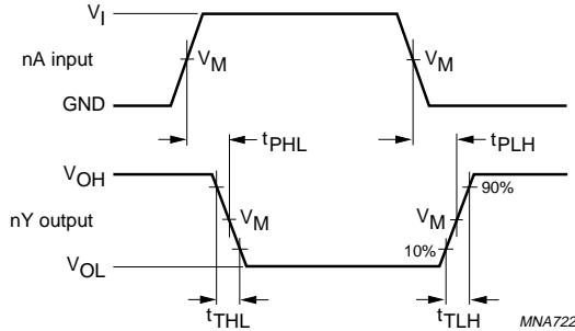
For 74HC04:  $V_M = 50\%$ ;  $V_I = GND$  to  $V_{CC}$ .For 74HCT04:  $V_M = 1.3 \text{ V}$ ;  $V_I = GND$  to  $3.0 \text{ V}$ .
