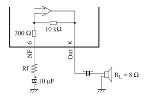
Bass boost can be easily implemented by inserting a series connection of RC between Pin8 (output) and Pin6 (NF). Example : Rb =  $12 \text{ k}\Omega$ , Cb =  $0.022 \,\mu\text{F}$
