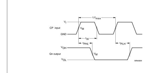
$V_M$  = 1.5 V at  $V_{CC} \ge 2.7$  V.
