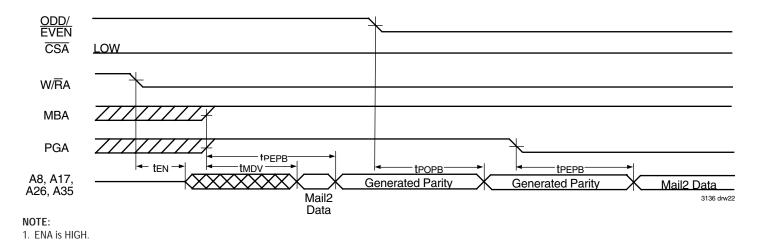
Figure 19. Parity Generation Timing when Reading from Mail2 Register
