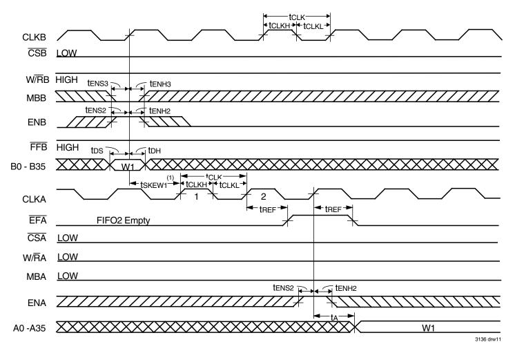
1. tskew1 is the minimum time between a rising CLKB edge and a rising CLKB edge for EFA to transition HIGH in the next CLKA cycle. If the time between the rising CLKB edge and rising CLKA edge is less than tskew1, then the transition of EFA HIGH may occur one CLKA cycle later than shown.
