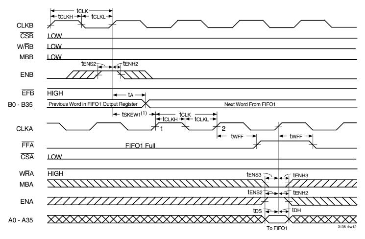
1. tskew1 is the minimum time between a rising CLKB edge and a rising CLKB edge for FFA to transition HIGH in the next CLKA cycle. If the time between the rising CLKB edge and rising CLKA edge is less than tskew1, then FFA may transition HIGH one CLKA cycle later than shown.
