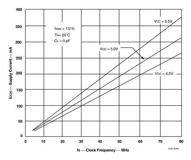
Figure 1. Typical Characteristics: Supply Current vs Clock Frequency
