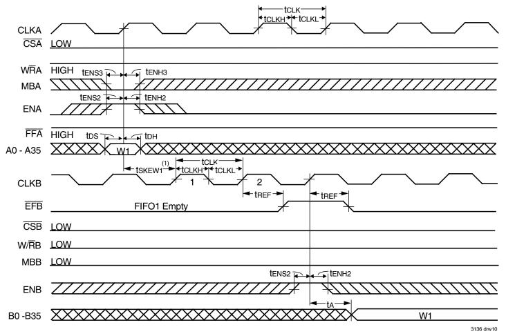
1. tskew1 is the minimum time between a rising CLKA edge and a rising CLKB edge for EFB to transition HIGH in the next CLKB cycle. If the time between the rising CLKA edge and rising CLKB edge is less than tskew1, then the transition of EFB HIGH may occur one CLKB cycle later than shown.
