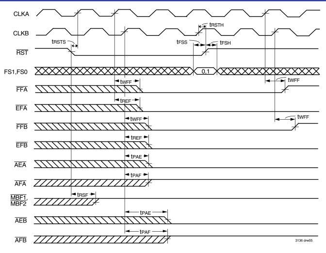
Figure 2. Device Reset Loading the X Register with the Value of Eight
