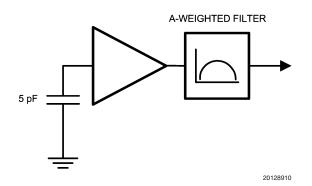
FIGURE 3. Noise Measurement Setup
