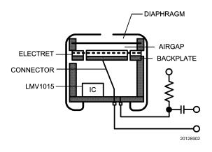
FIGURE 1. Built in Gain
