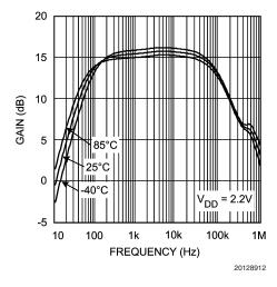
FIGURE 5. LMV1015-15 Gain vs. Frequency Over Temperature
