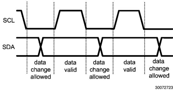
FIGURE 6. I<sup>2</sup>C Signals: Data Validity
