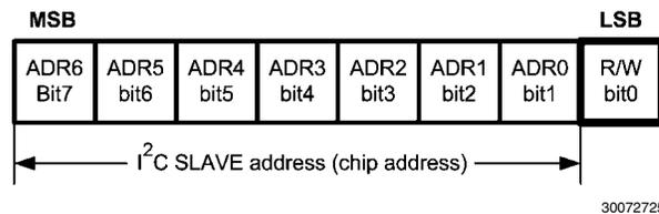
FIGURE 8. I<sup>2</sup>C Chip Address
