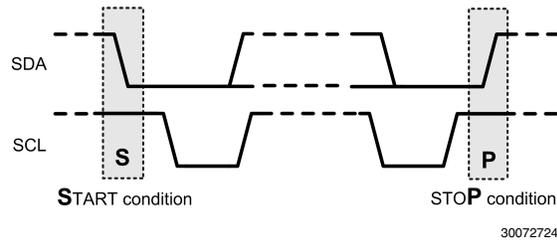
FIGURE 7. I<sup>2</sup>C Start and Stop Conditions
