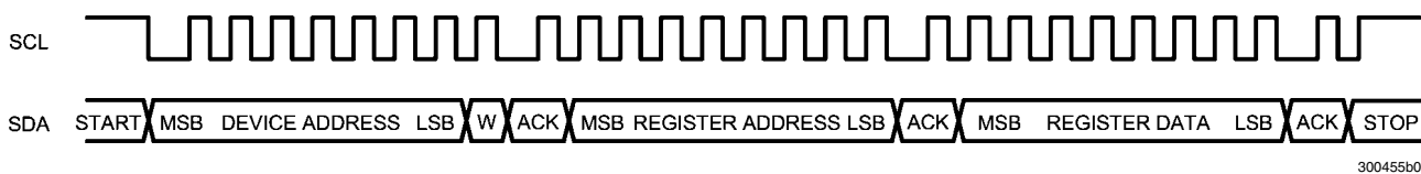
FIGURE 4. Example I 2 C Write Cycle
