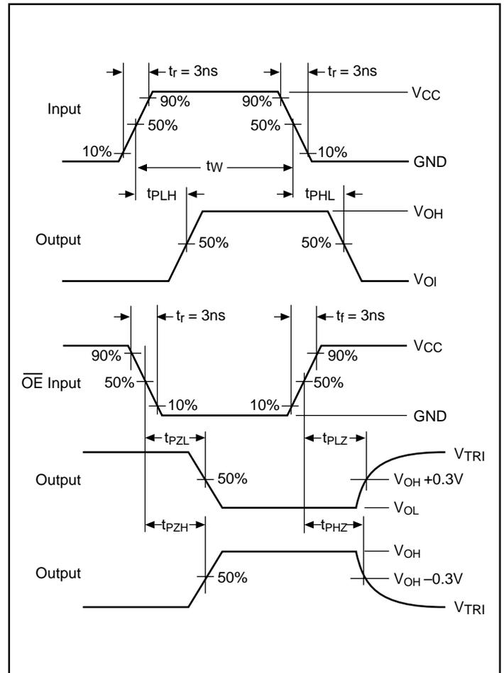
Figure 3. AC Waveforms
