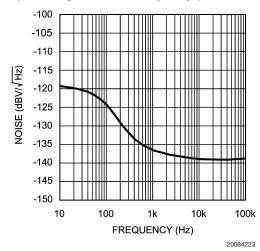
Output Voltage Noise vs. Frequency (LMV1032-25)
