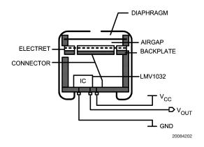
FIGURE 1. Built-in Gain
