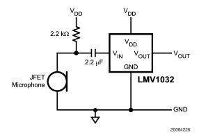
FIGURE 6. LMV1032 as External Pre-Amplifier
