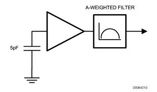
FIGURE 3. Noise Measurement Setup
