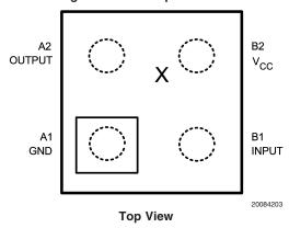
Note: - Pin numbers are referenced to package marking text orientation.
