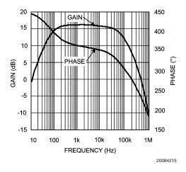
FIGURE 5. Gain vs. Frequency
