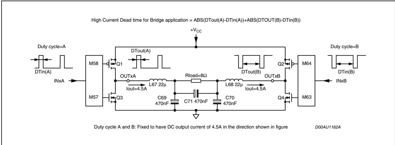
Figure 7. Typical Single BTL Configuration to Obtain 80W @ THD 10%,  $R_L = 8\Omega$ ,  $V_{CC} = 36V$  (note 1)
