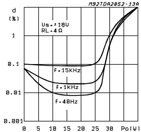
Figure 5: Distortion vs. Frequency.
