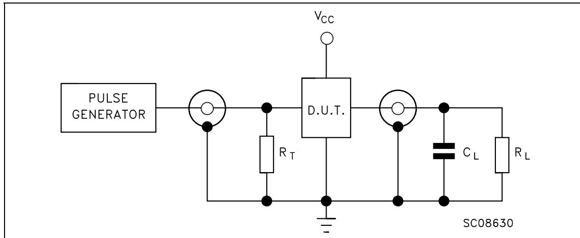
**TEST CIRCUIT AND WAVEFORM SYMBOL VALUE**
