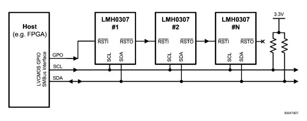
FIGURE 2. SMBus Configuration for Multiple LMH0307 Cable Drivers
