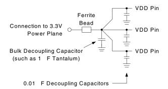
All power supply pins must be connected to the same voltage, except VDDO, which may be connected to a lower voltage in order to change the output level.
