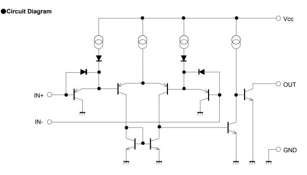
Fig.1 Circuit Diagram (each Comparator)
