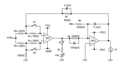
Fig.2 Measurement Circuit1 (each Comparator)
