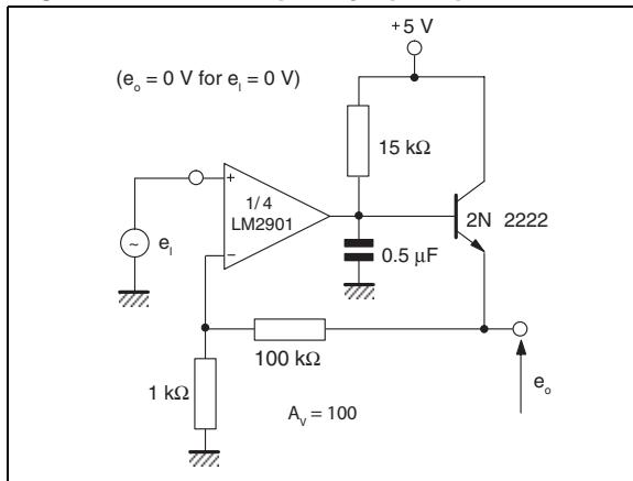
Figure 12. Transducer amplifier
