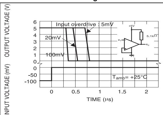
**Figure 6. Response time for various input overdrives - positive transition**
