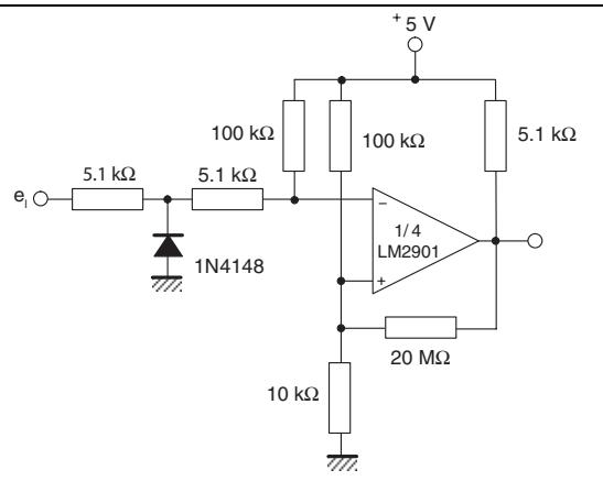
**Figure 16. Split-supply applications - zero crossing detector**
