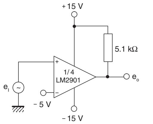
Figure 19. Time delay generator
