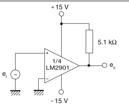
**Figure 18. Comparator with a negative reference**
