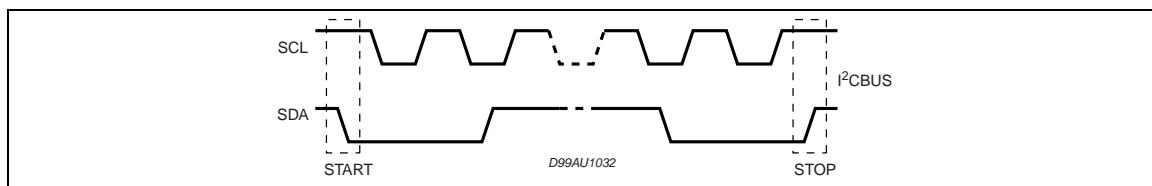
**Figure 7. Acknowledge on the I<sup>2</sup>CBUS**
