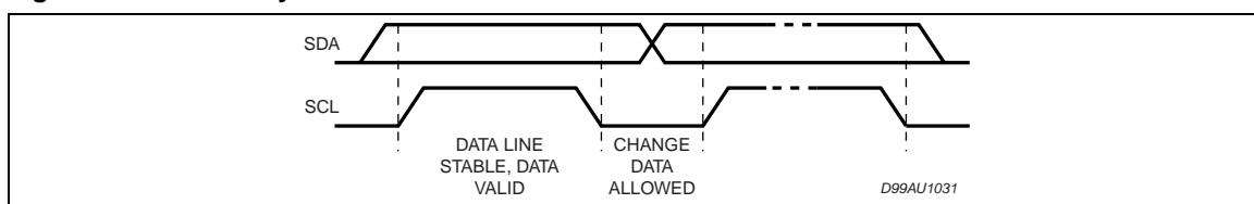
**Figure 6. Timing Diagram of I<sup>2</sup>CBUS**
