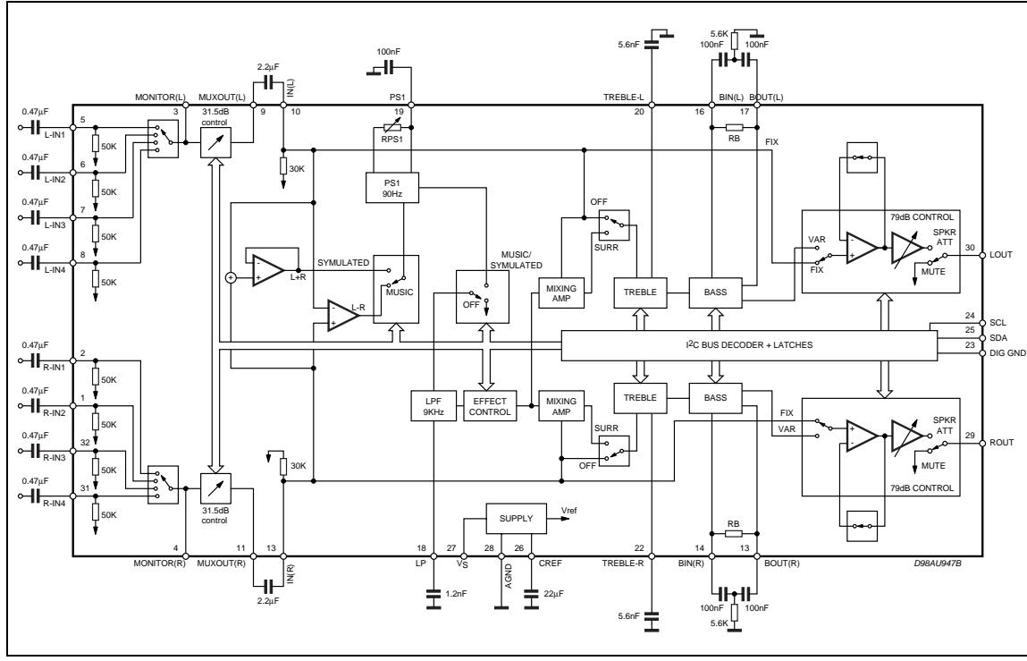
**Figure 4. Block Diagram (TDA7442D)**
