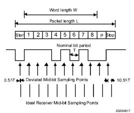
FIGURE 15. Deviated Baud Rate Sampling
