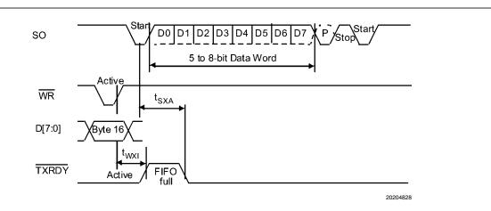
FIGURE 26. Transmitter Timing FIFO Mode
