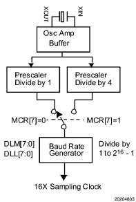
**FIGURE 1. Internal Clock Dividers**
