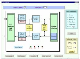
The FALC Configuration Assistant supports the user during design phase. All DualFALC functional blocks can be configured by a GUI supporting the low level API driver.
