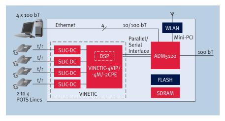
VoIP Router and ATA Application Example for One Hardware for All "Voice over Packet" Applications
