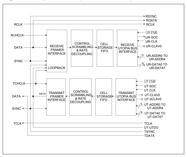
Figure 2-6. Backplane Interface (UTOPIA Bus Enabled)
