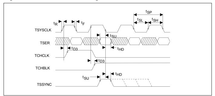
Figure 36-12. Transmit-Side Timing, Elastic Store Enabled
