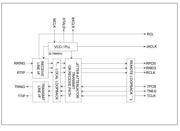
Figure 2-3. Receive and Transmit LIU (UTOPIA Backplane Enabled)
