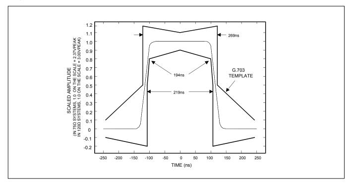
Figure 23-6. T1 Transmit Pulse Template
