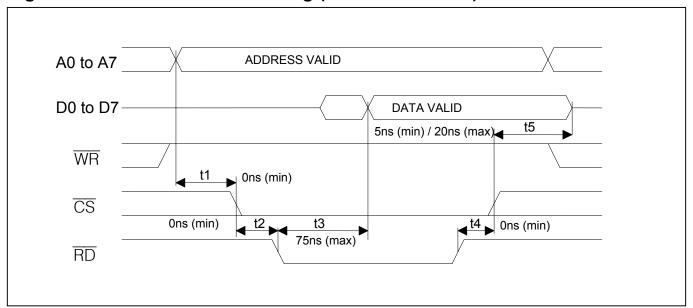
Figure 36-4. Intel Bus Read Timing (BTS = 0/MUX = 0)
