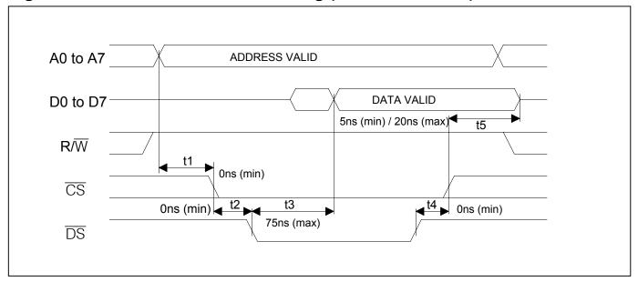
Figure 36-6. Motorola Bus Read Timing (BTS = 1/MUX = 0)
