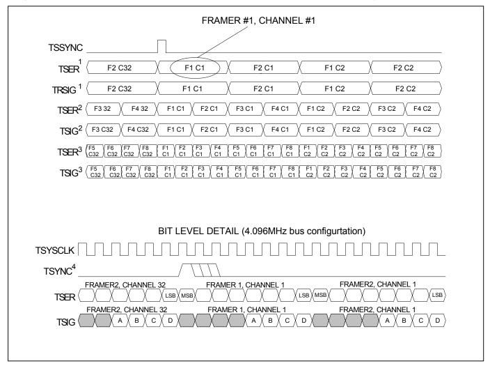
Figure 34-22. Transmit IBO Channel Interleave Mode Timing
