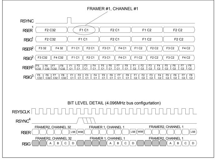
Figure 34-15. Receive IBO Channel Interleave Mode Timing
