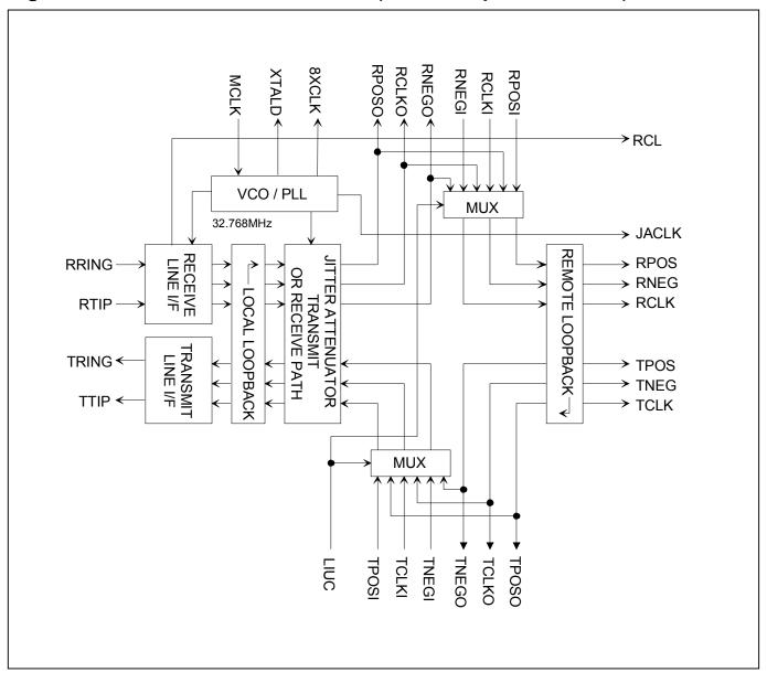
Figure 2-2. Receive and Transmit LIU (TDM Backplane Enabled)
