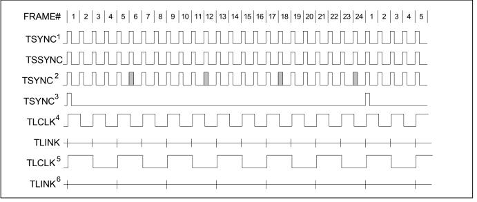
Note 1: TSYNC in frame mode (IOCR1.2 = 0) and double-wide frame sync is not enabled (IOCR1.3 = 0).
