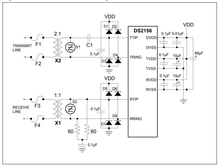
Figure 23-4. Protected Interface Using Internal Receive Termination
