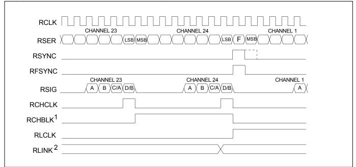
Figure 34-3. Receive-Side Boundary Timing (with elastic store disabled)
