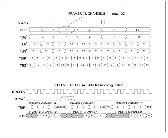
Figure 34-23. Transmit IBO Frame Interleave Mode Timing
