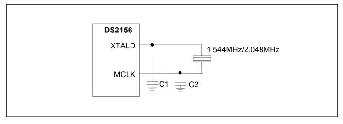
Note 1: C1 and C2 should be 5pF lower than two times the nominal loading capacitance of the crystal to adjust for the input capacitance of the DS2156.
