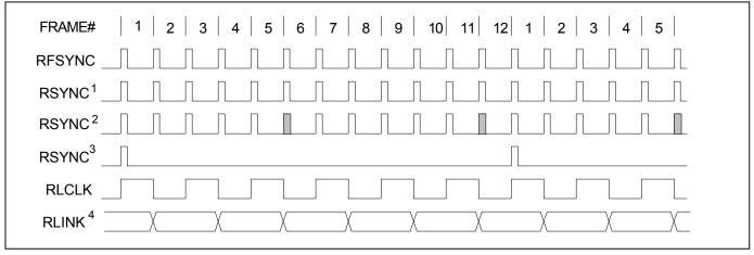
Note 1: RSYNC in the frame mode (IOCR1.5 = 0) and double-wide frame sync is not enabled (IOCR1.6 = 0).
