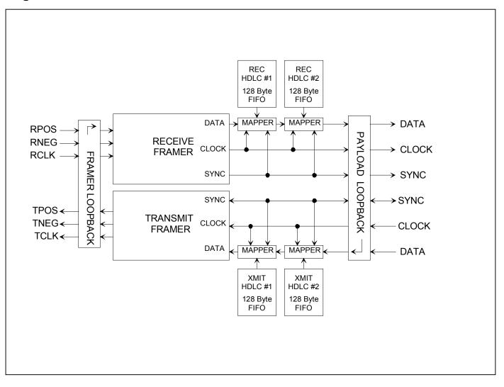
Figure 2-4. Receive and Transmit Framer/HDLC
