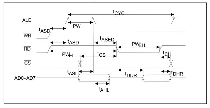
Figure 36-1. Intel Bus Read Timing (BTS = 0/MUX = 1)
