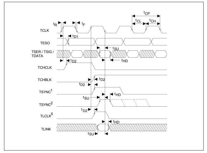
Note 1: TSYNC is in the output mode (IOCR1.1 = 1).
