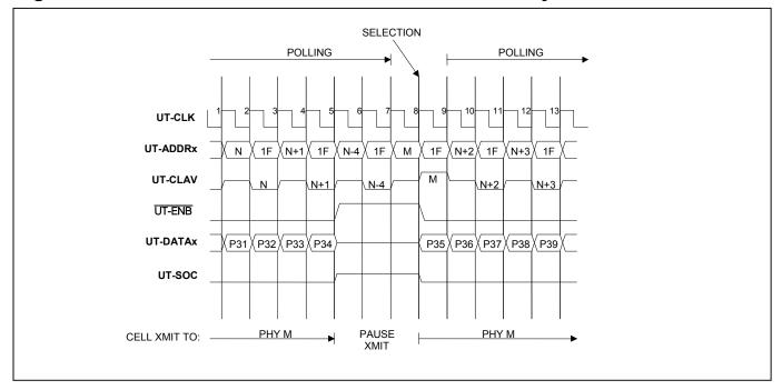
Figure 24-4. Transmission to PHY Paused for Three Cycles
