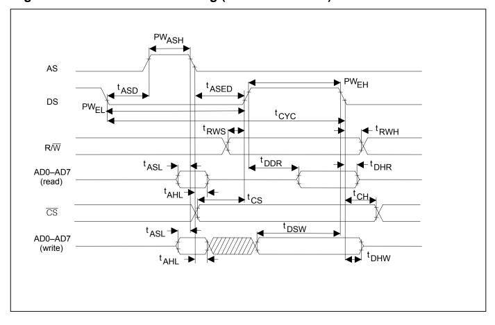
Figure 36-3. Motorola Bus Timing (BTS = 1/MUX = 1)
