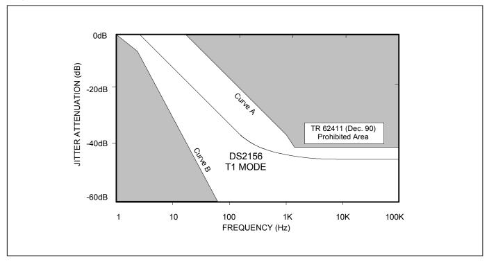
Figure 23-9. Jitter Attenuation (T1 Mode)
