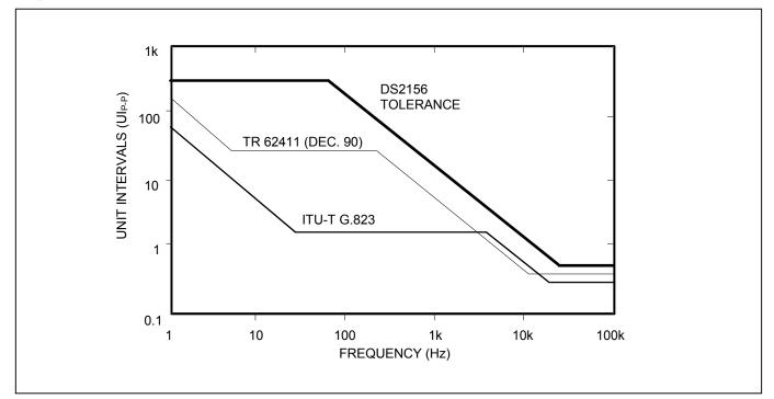
Figure 23-8. Jitter Tolerance (E1 Mode)
