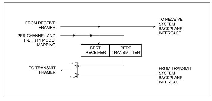
Figure 26-1. Simplified Diagram of BERT in Network Direction
