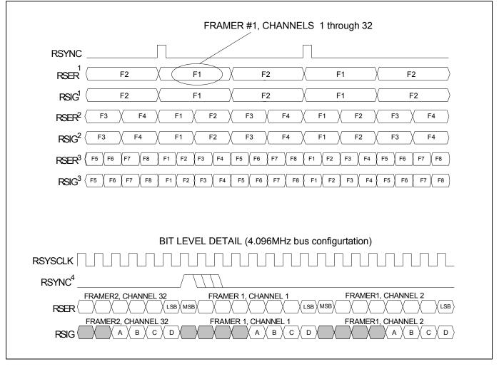
Figure 34-16. Receive IBO Frame Interleave Mode Timing
