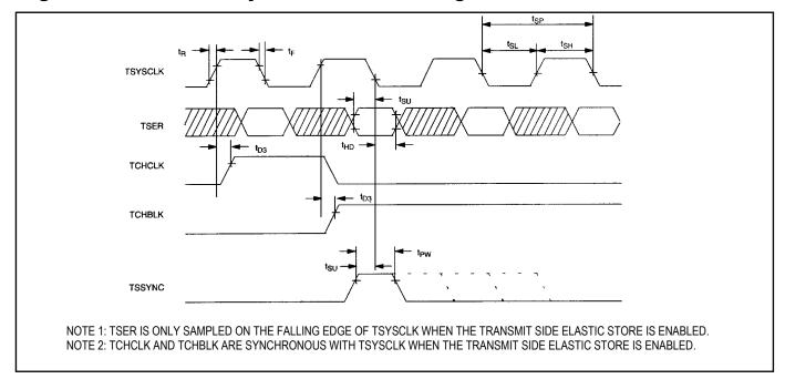
Figure 18-8. Transmit System Side AC Timing
