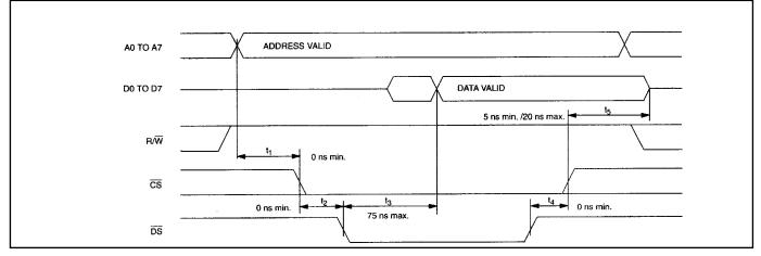
Figure 18-13. Motorola Bus Write AC Timing (BTS = 1/MUX = 0)
