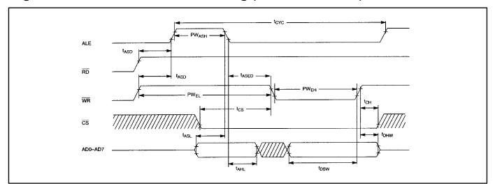
Figure 18-3. Motorola Bus AC Timing (BTS = 1/MUX = 1)
