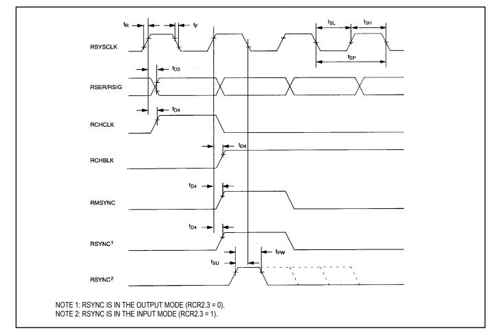
Figure 18-5. Receive System Side AC Timing
