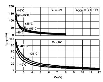
FIGURE 15. ENABLE TURN - OFF TIME vs SUPPLY VOLTAGE
