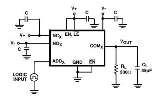
Repeat test for other switches. C<sub>L</sub> includes fixture and stray capacitance.
