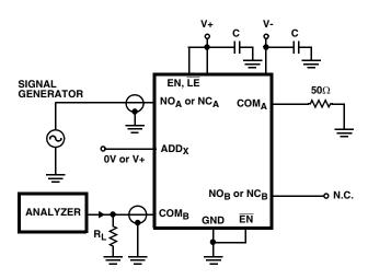
FIGURE 7. CROSSTALK TEST CIRCUIT
