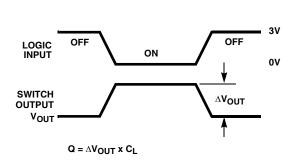
FIGURE 2A. Q MEASUREMENT POINTS
