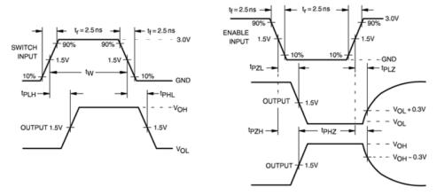
Figure 4. AC Waveforms
