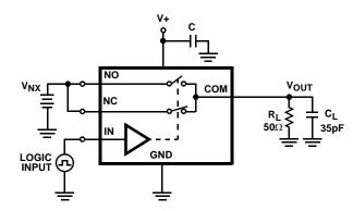
NOTE:  $C_L$  INCLUDES FIXTURE AND STRAY CAPACITANCE. FIGURE 3B. TEST CIRCUIT
