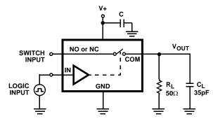
NOTE: REPEAT TEST FOR ALL SWITCHES.  $\mathbf{C}_{L}$  INCLUDES FIXTURE AND STRAY CAPACITANCE.
