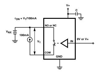
FIGURE 5. ron TEST CIRCUIT
