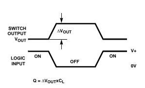
FIGURE 2A. MEASUREMENT POINTS
