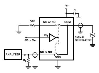
FIGURE 6. CROSSTALK TEST CIRCUIT
