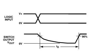
FIGURE 3A. MEASUREMENT POINTS
