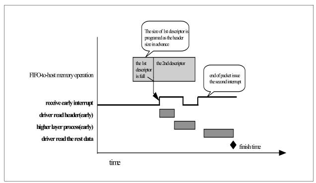
Figure 13 Detailed Receive Early Interrupt Flow
