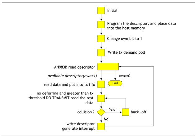
Figure 9 Transmit Flow
