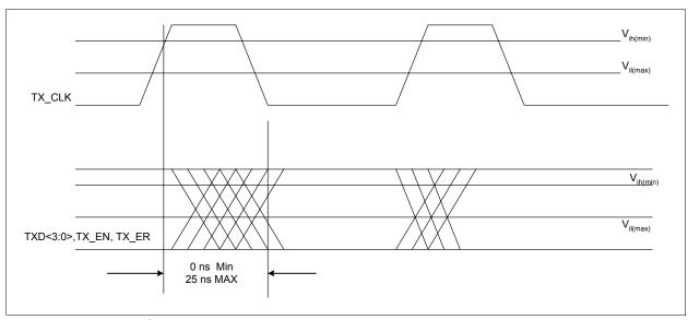
Figure 21 Transmit Signal Timing Relationships at the MII
