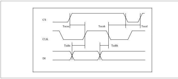
Figure 20 Serial EEPROM Timing
