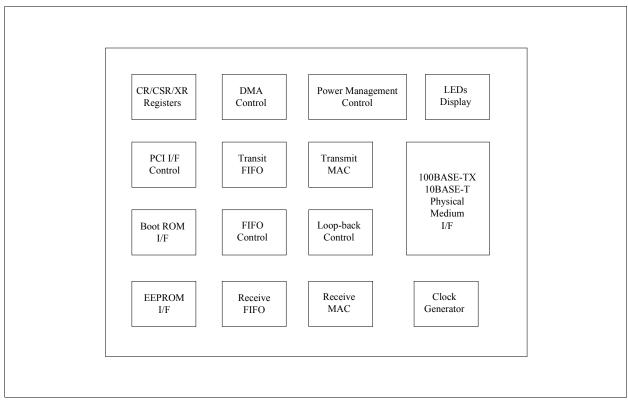
Figure 2 Block Diagram of the AN983B/BX
