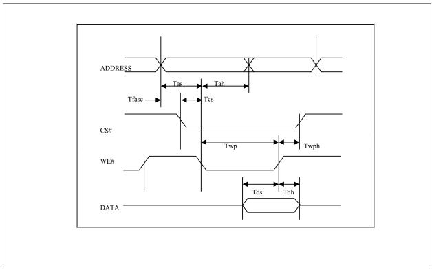
Figure 18 Flash Write Timings
