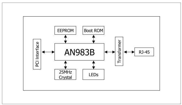
Figure 1 System Diagram of the AN983B/BX
