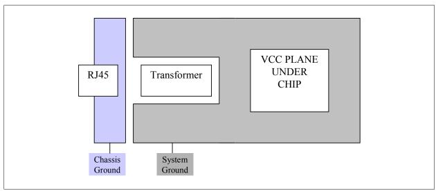
Figure 28 Ground Plane Arrangement
