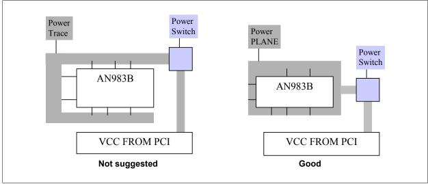
Figure 27 Power Trace Arrangement
