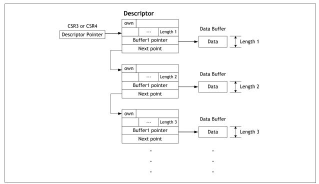
Figure 6 Chain Structure of Frame Buffer
