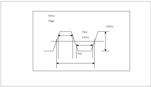
Figure 16 PCI Clock Waveform
