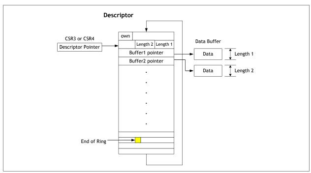
Figure 5 Ring Structure of Frame Buffer
