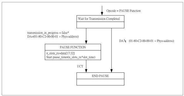
Figure 15 PAUSE Operation Receive State Diagram
