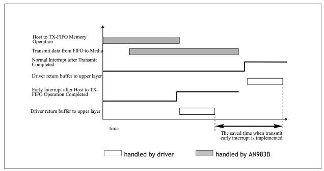
Figure 11 Transmit Normal Interrupt and Early Interrupt Comparison
