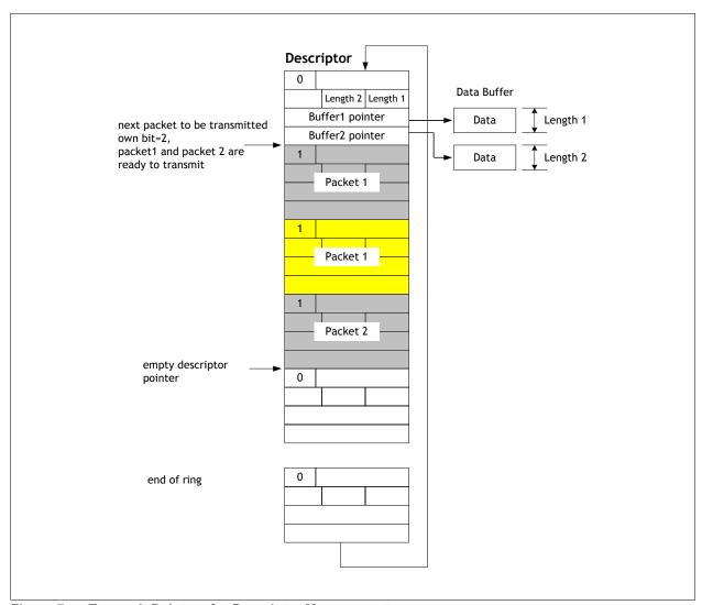
Figure 7 Transmit Pointers for Descriptor Management
