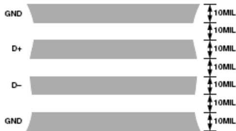
Figure 16. Arrangement of Signal Tracks
