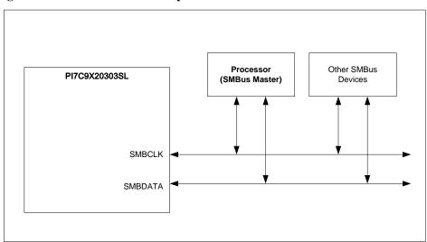
Figure 6-1 SMBus Architecture Implementation on PI7C9X20303SL
