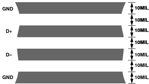
Figure 18. Arrangement of Signal Tracks
