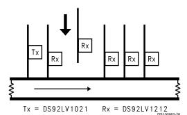
The DS92LV1212 can be "Hot Inserted" into operating serial busses without interrupting bus communication. The random lock feature allows the DS92LV1212 to synchronize to the bus traffic and receive data.
