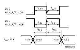
Timing shown for RCLK\_R/ $\overline{F}$  = LOW Duty Cycle (t<sub>RDC</sub>) =  $\frac{t_{HIGH}}{t_{HIGH}} + t_{IIOW}$
