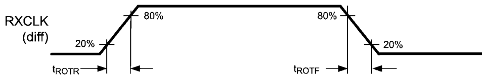
FIGURE 2. LVDS Output Transition Time
