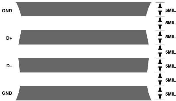
Figure 16. Typical Arrangement of Signal Tracks
