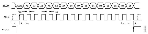
Figure 8. Serial Write Operation Timing
