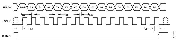
Figure 9. Serial Read Operation Timing
