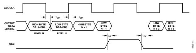
Figure 7. Digital Output Data Timing
