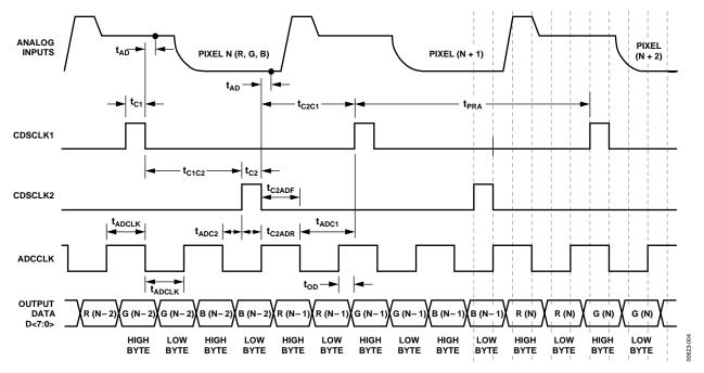
Figure 3. 3-Channel CDS Mode Timing
