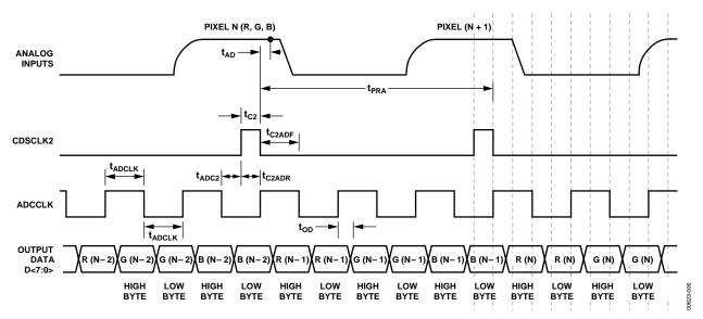
Figure 5. 3-Channel SHA Mode Timing
