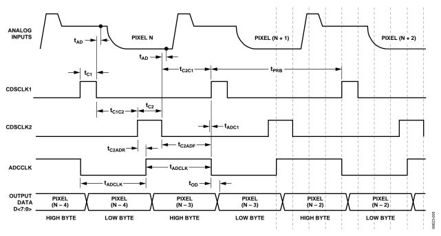
Figure 4. 1-Channel CDS Mode Timing
