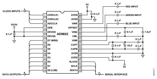
Figure 16. Recommended Circuit Configuration, 3-Channel CDS Mode
