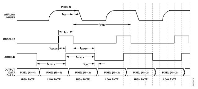
Figure 6. 1-Channel SHA Mode Timing
