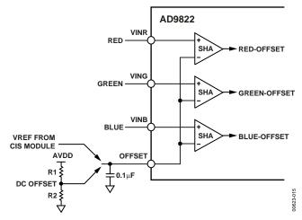
Figure 14. SHA Mode Used with External DC Offset
