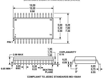
Figure 19. 28-Lead Shrink Small Outline Package [SSOP] (RS-28) Dimensions shown in millimeters
