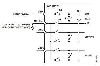
Figure 12. SHA Mode Input Configuration (All Three Channels are Identical)
