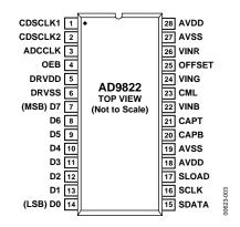
Figure 2. Pin Configuration
