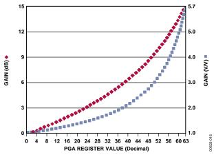
Figure 15. PGA Gain Transfer Function
