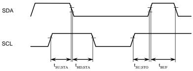
Figure 1 - 2-WIRE Start and Stop timings
