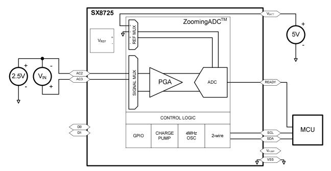
Figure 18 - Recommended Operation Mode Schematic
