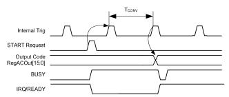
Figure 10 - ADC "On-Request" Operation
