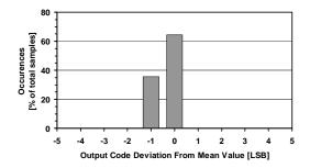
Figure 24 - ADC Noise (PGA1, 2 & 3 Bypassed, OSR = 512, N<sub>ELCONV</sub> = 2)
