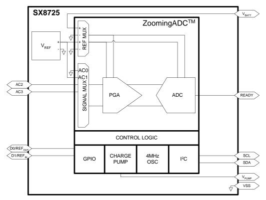
Figure 3 - SX8725 Block Diagram
