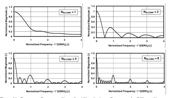
Figure 21 - Frequency Response: Normalized Magnitude vs. Frequency for Different N<sub>ELCONV</sub>
