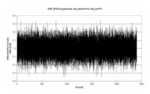
Figure 23 - Differential Non-Linearity of the ADC Converter
