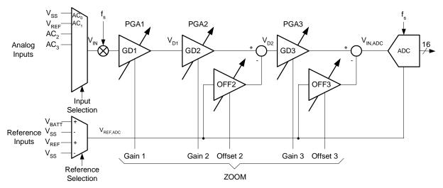
Figure 8 - ZADC General Functional Block Diagram
