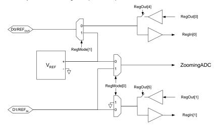
Figure 4 - GPIO Block Diagram
