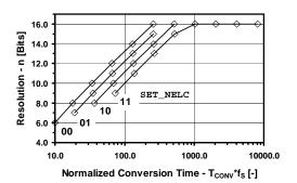
Figure 13 - Resolution vs. Normalized Conversion Time for Different SET\_NELC[1:0]
