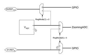
Figure 14 - D0 and D1 are Digital Inputs / Outputs
