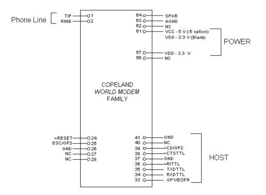
Note: Signals on pins 24, 25, 33-40 are TTL.
