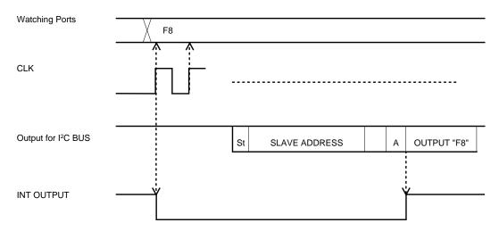
In the case that there is a change in detection ports once, and there are another changes before returning the ACK (as shown "A term"), then watching data is saved. And the output data in this case will be "AND" output of every bits of the watching data.
