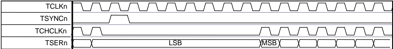
Figure 11-31. E1 Transmit-Side TCHCLKn Gapped Mode During Channel 1
