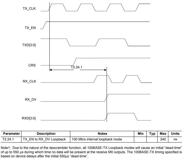
Note2: Measurement is made from the first rising edge of TX CLK after assertion of TX EN.
