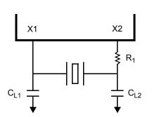
Figure 12. Crystal Oscillator Circuit
