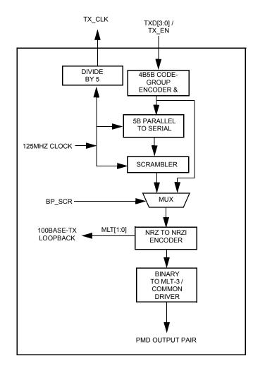
Figure 6. 100BASE-TX Transmit Block Diagram
