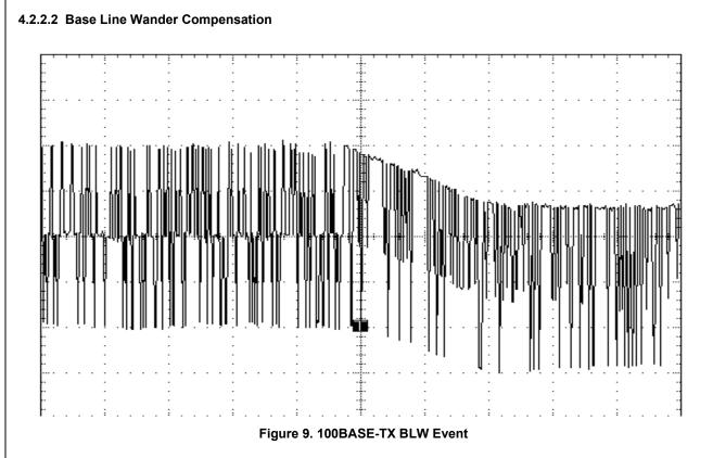
The DP83848C is completely ANSI TP-PMD compliant and includes Base Line Wander (BLW) compensation. The BLW compensation block can successfully recover the TP-PMD defined "killer" pattern.
