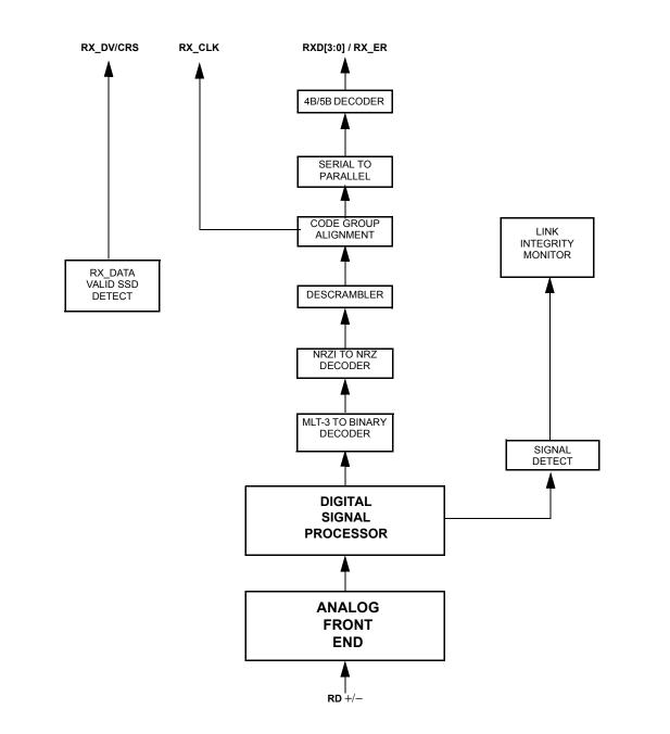
Figure 7. 100BASE-TX Receive Block Diagram
