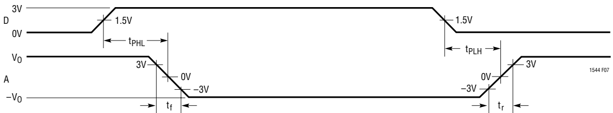
Figure 7. V.10, V.28 Driver Propagation Delays
