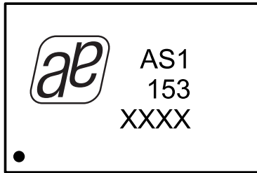
Figure 22. 8-pin SOIC Marking
