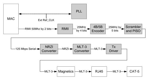
Figure 3.1 100BASE-TX Transmit Data Path
