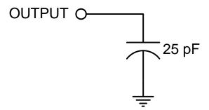
Figure 5.1 Output Equivalent Test Load
