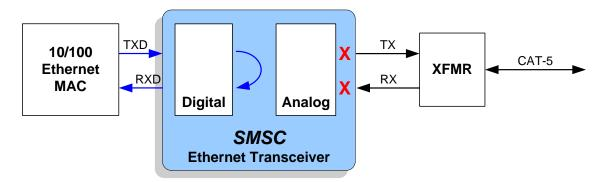
Figure 3.12 Near-end Loopback Block Diagram
