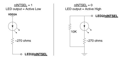
Figure 3.11 LED2/nINTSEL Polarity Configuration
