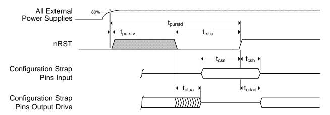
Figure 5.3 Power-On nRST & Configuration Strap Timing
