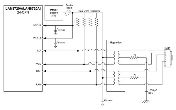
Figure 3.18 Twisted-Pair Interface Diagram (Single Power Supply)
