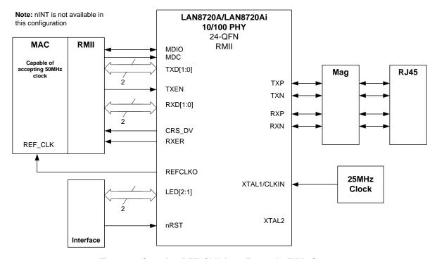
Figure 3.9 Sourcing REF\_CLK from External 25MHz Source
