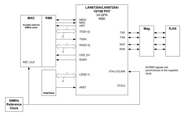
Figure 3.7 External 50MHz clock sources the REF\_CLK
