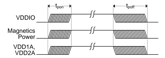
Figure 5.2 Power Sequence Timing
