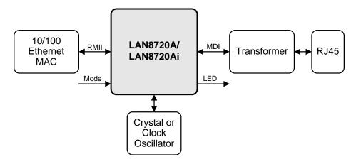
Figure 1.1 System Block Diagram
