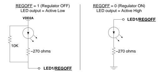
Figure 3.10 LED1/REGOFF Polarity Configuration
