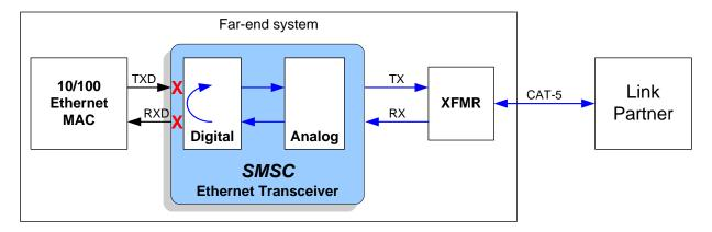
Figure 3.13 Far Loopback Block Diagram
