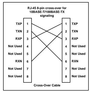
Figure 3.4 Direct Cable Connection vs. Cross-over Cable Connection
