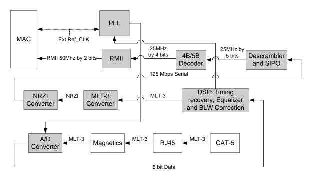
Figure 3.2 100BASE-TX Receive Data Path
