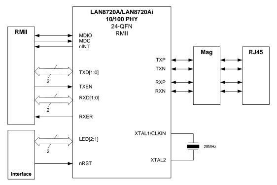
Figure 3.15 Simplified System Level Application Diagram
