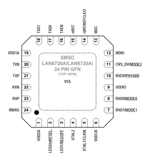
NOTE: Exposed pad (VSS) on bottom of package must be connected to ground
