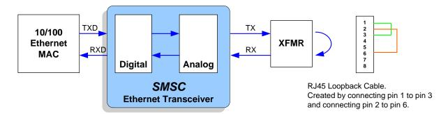
Figure 3.14 Connector Loopback Block Diagram
