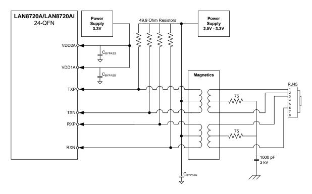
Figure 3.19 Twisted-Pair Interface Diagram (Dual Power Supplies)
