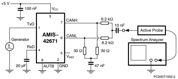
Figure 8. Basic Test Setup for Electromagnetic Measurement
