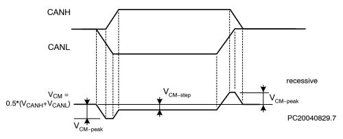
Figure 9. Common-Mode Voltage Peaks (see Measurement Setup Figure 8)
