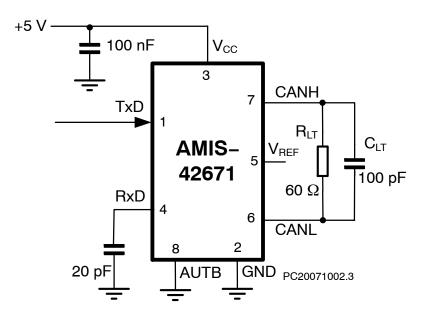
Figure 6. Test Circuit for Timing Characteristics
