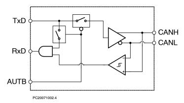
Figure 3. Simplified Schematic Diagram of Autobaud Function
