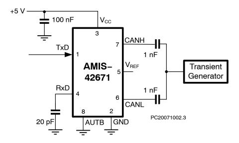
Figure 4. Test Circuit for Transients
