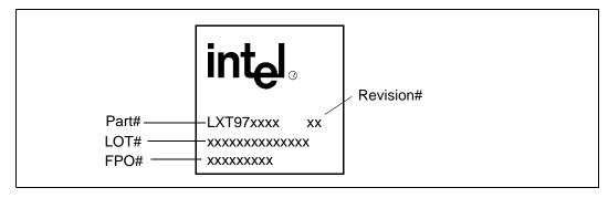
The silicon stepping in the LXT97xx Data Sheets is referred to as "Manufacturer's Revision Number." The silicon stepping number may be read by software from Register 3, bits 3:0 in the LXT97xx transceivers.
